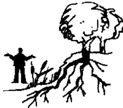
Trees contribute cohesion and stability to steep banks- Providing the roots reach down to full bank height and the toe- hold and bank-face are protected from undercutting by tree roots and an established cover
