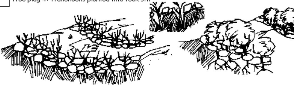
Tree plug 5: Truncheons planted alongside a roll gabion sill filled with rock and soil
