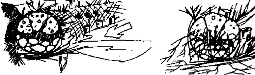
☐ Herbaceous 8: Root clumps of grass, sedge, reed or bulrush planted in standard gabions or containers and anchored into trenches with stakes
