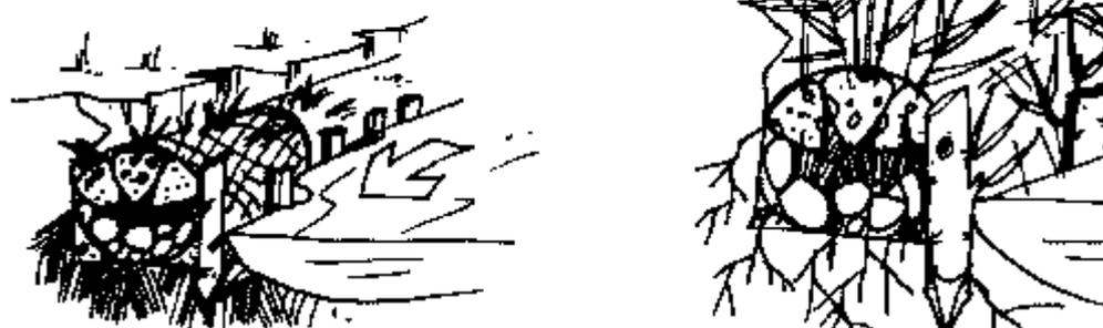
Herbaceous 7: Root clumps of grass, sedge, reed or bulrush planted in roll gabions placed over silt trap layer of dead branches, and anchored into trenches with stakes
