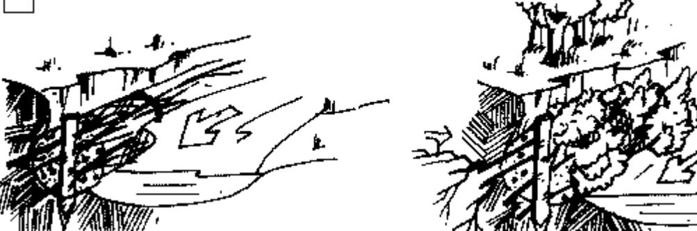
7. Tree truncheons laid into front and top of gabions or concertainers filled with stone soil.
