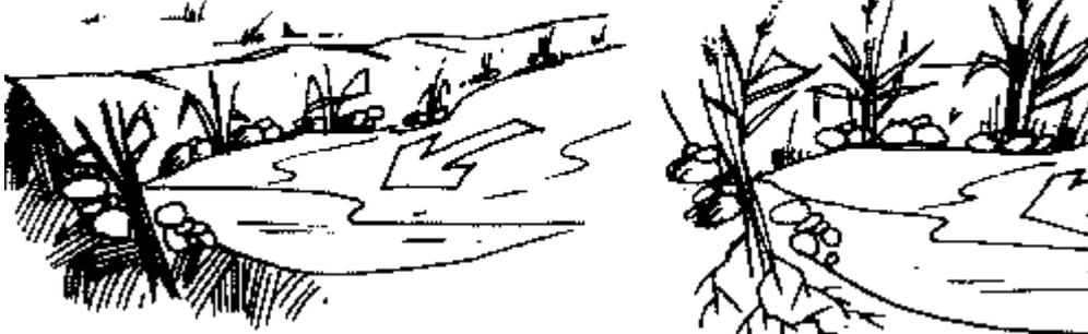
Herbaceous 6: Root clumps of grass, sedge, reed or bulrush planted in roll gabions anchored into trenches with stakes
