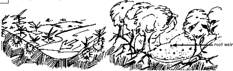
Tree plug 3: Truncheons ground layered into the channel
